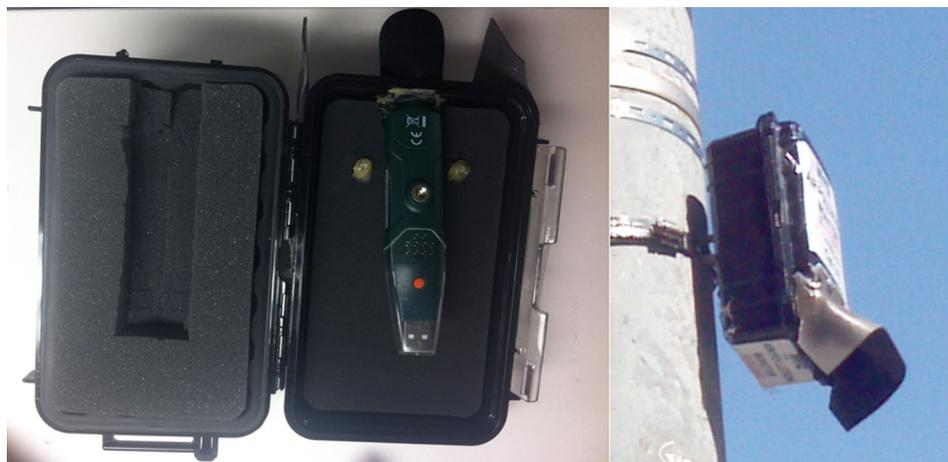
**FIGURE 1.** Community noise monitor field deployment and housing design.
